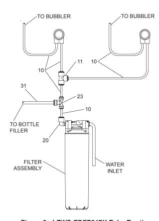
Figure 3 - LZWS-EDFP217K Tube Routing
