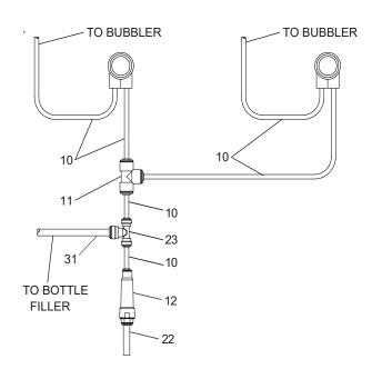
Figure 2 - EZWS-EDFP217K Tube Routing
