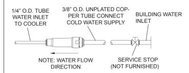
Figure 10 - Water Supply Connections
