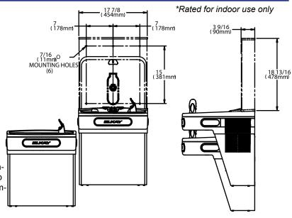
Bottle Filler unit will mount on bracket attached to wall by 6 holes (as shown). Water and electrical will connect through pre-punched hole in basin.
