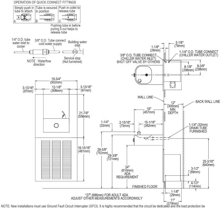
NOTE: New installations must use Ground Fault Circuit Interrupter (GFCI). It is highly recommended that the circuit be dedicated and the load protection be sized for 20 amps.
