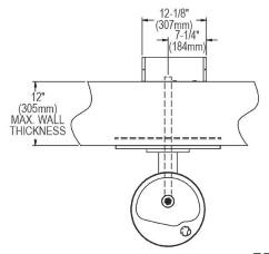
WARNING: The free-resistant box must be installed on an interior heated wall where the temperature does not drop below 50° F (10° C). The front of the box must have unobstructed air flow. Failure to maintain the interior wall temperature and the inside of the freeze resistant box above 50° F (10° C) can result in damage to the box which could result in unrestricted
