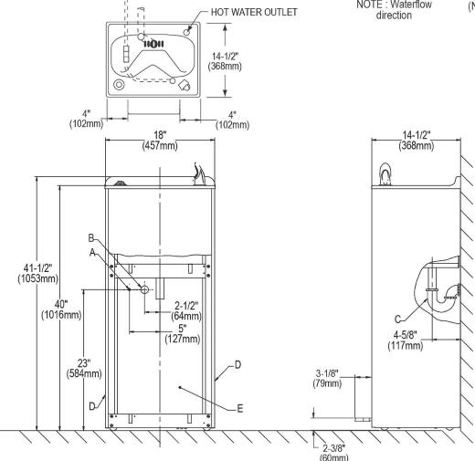
A = Recommended water supply location 3/8" O.D. unplated copper tube connect stub out 1-1/2" (38mm) from wall shut off by others. B = Recommended location for waste outlet 1-1/4" O.D. drain.
