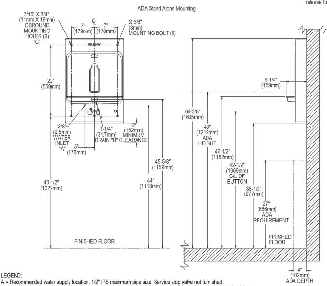
B = Recommended waste location. Waste shown in wall but may be behind wall outlet 1-1/4" O.D. (Trap not furnished).
