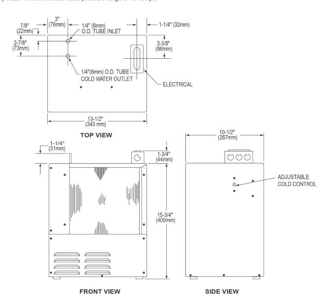
NOTE: It is important to insure proper ventilation. Allow a minimum clearance of 6" (152 mm) in front and 3"(76 mm) in the rear of the unit. If unit is to be installed in an enclosure, allow the following clearances around unit: 1"(25 mm) each side, 3"(76 mm) in the rear, 3"(76 mm) above.
