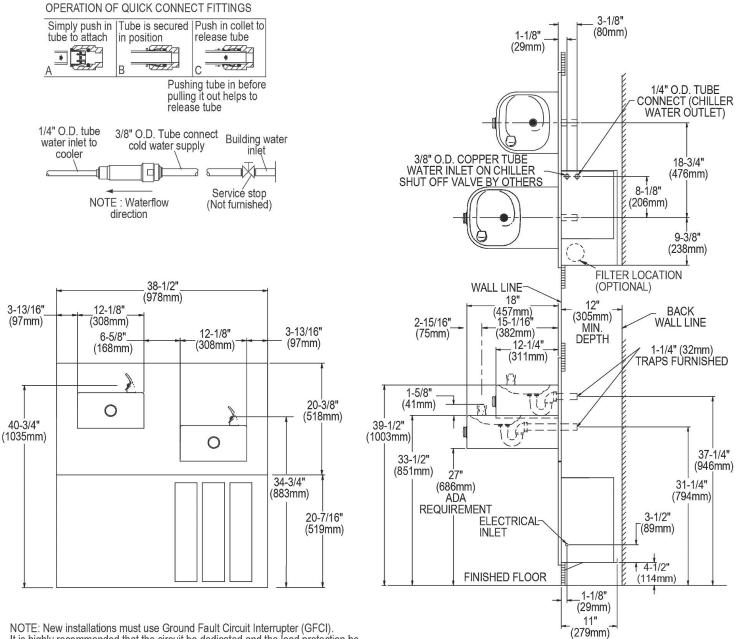
It is highly recommended that the circuit be dedicated and the load protection be sized for 20 amps.
