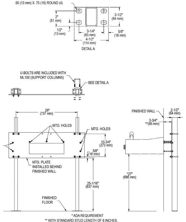
NOTE - AFTER INSTALLATION, U-BOLTS AND THREADED RODS MAY NEED TO BE TRIMMED
