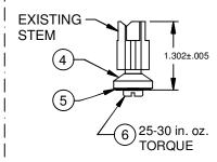
SEAT & OPERATOR STEM ASSEMBLY DETAIL
