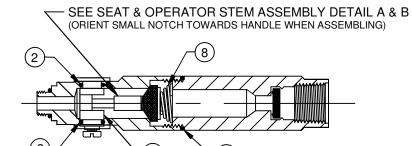
CLEAN VALVE THOROUGHLY AND LUBRICATE 'O' RINGS WITH 'O' RING LUBE BEFORE REASSEMBLING.
