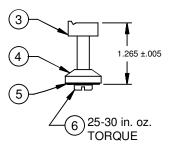
SEAT & OPERATOR STEM ASSEMBLY DETAIL
