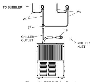
Figure 3 - ERPB Tube Routing
