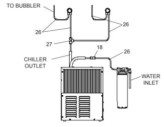
Figure 4 - LRPB Tube Routing
