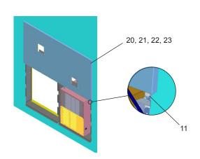
Figure 5 - Upper Panel Installation
