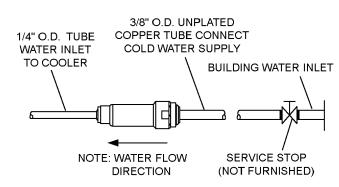
Figure 12 - Water Supply Connections
