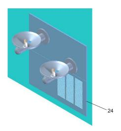
Figure 7 - Lower Panel Installation
