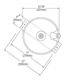
NOTE: Rough-in dimensions may vary 1/2" (13mm) ±. Rubber can be mounted on right or left as desired.
