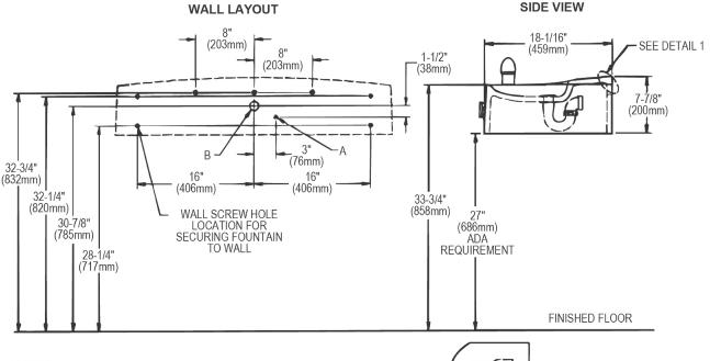
A = 3/8" O.D. tube connect - shut off valve by others B = Water outlet 1-1/4" O.D. drain-stub out from wall 1" (25mm)
