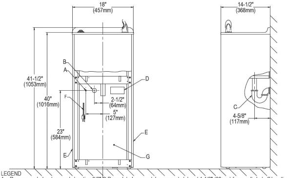
A = Recommended water supply location 3/8" O.D. unplated copper tube connect stub out 1-1/2" (38mm) from wall shut off by others.
