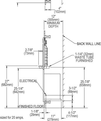
Note: New Installations Must Use Ground Fault Circuit Interrupter (GFCI). It is highly recommended that the circuit be dedicated and the load protection be sized for 20 amps.
