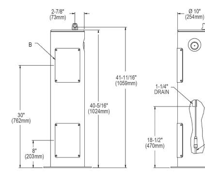
A = 3/8" O.D. UNPLATED COPPER TUBE CONNECT SHUT OFF VALVE BY OTHERS B = ACCESS PANEL (8" x 10")
