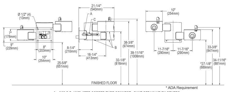
A = 3/8" O.D. UNPLATED COPPER TUBE CONNECT - SHUT OFF VALVE BY OTHERS
