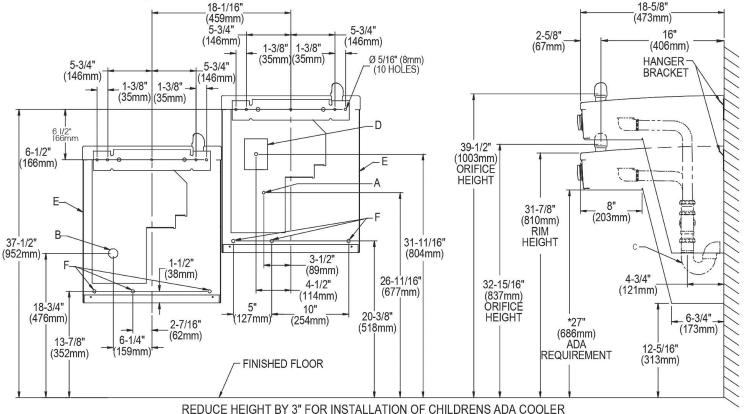
A = Recommended water supply location. Shut off valve (not furnished) to accept 3/8" O.D. unplated copper tube. 3" (76mm) maximum out from wall. B = Recommended location for waste outlet 1-1/2" O.D. drain. Drain stub 2" (51mm) out from wall.
