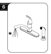
Important: After installation is completed, remove aerator assembly. Turn on hot and cold water supplies. Turn handle to full open position for one minute. Check for leaks. Replace aerator.
