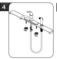
Place faucet in position on sink. From under sink, screw mounting nuts onto faucet. Tighten mounting nuts. Hand tighten only.
