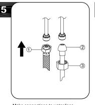
Make connections to water lines. Use 1/2" I.P.S. faucet connections (1) or use coupling nuts (3) with 3/8" O.D.ball-nose riser(2). Use wrenches to tighten connections. Do not overtighten.
