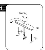
Shut off water supplies. Screw bolt (1) onto the escutcheon (2). If your model has a spray, proceed to step 2. If your model does not have a spray, skip to step 4.
