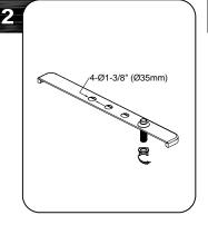
For models with spray (fits 4 - hole sinks): Insert spray support through far right - hand hole on sink. Screw hold - down nut onto shank and hand tighten.
