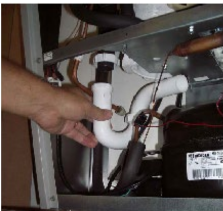
Loosen Drain Line
