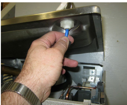
Remove Bubbler Water Line
