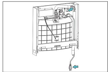
6. Feed the power cord and water line through hole on top of the water cooler.
