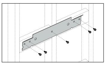
4. Hang unit onto the hanger bracket.
