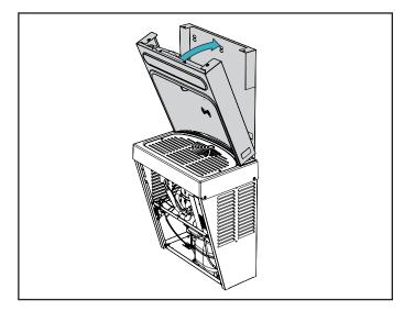
9. Slide the bottle filler down to nest in place. Rib on the basin should be behind the bottle filler alcove.
