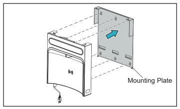
Place mounting plate against wall on top of the basin. Center the mounting plate side to side with the basin. Mark the six (6) mounting holes with a pencil.
