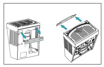
5. Install the two mounting screws to attach cooler to the wall.
