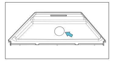
3. Trial fit the strainer. If the strainer does not fit, carefully open the size of the hole. If it fits well, place a small amount of plumbers putty around the lip of the strainer flange and insert it into the hole. If the flange does not fit, carefully open the size of the hole.
