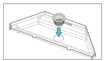
4. Install the O-ring over the strainer threads.
