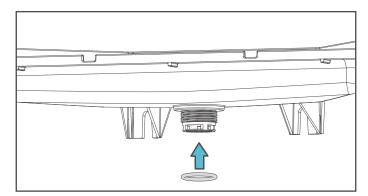
Thread the strainer into the drain adapter.
