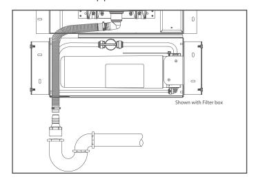
9. Connect the drain adapter into the household waste drain pipe.
