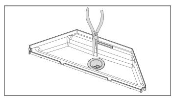
Attach one end of the 3/4 inch flexible drain hose to the 3/4 inch barbed drain adapter connection using the supplied hose clamp. The supplied flexible drain is 13 inches long. If a longer drain hose is required, it must be installer-supplied.
