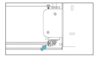
3. Connect an installer supplied 3/8 inch water supply tube to the quarter-turn shutoff valve, as shown. The type of tubing, copper or plastic, should meet all local regulations and building codes.
