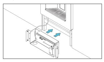
**Note:** Some side-to-side and up-and-down movement of the housing is capable to accurately align the filter unit with the water dispenser.
