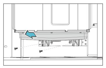
2. Place the drain basin on a flat, hard surface, such as a piece of sacrificial wood. Carefully drill a hole in the basin using a 1-inch hole saw using the centering-dimple as a guide to center the hole saw. Do not use a 1-1/8" hole saw as this will make the opening too large.
