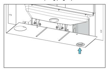
**Note:** The space behind that filter box is limited so make sure any electrical wiring will not interfere with mounting the filter box into the wall. Refer to "4.3 Critical Depth Dimensions" on page 8 for additional information.
