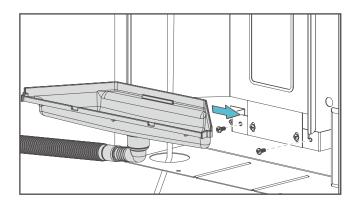
8. Route the drain hose through the filter box and attach the other end to the p-trap drain adapter using a hose clamp. The drain adapter is designed to be glued into a 1-1/4 inch PVC pipe.
