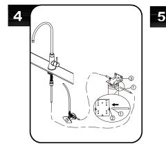
Connect the bottom of pipe (1) into the end (2) with outlet indicated of the filtration manifold (3). Pull moderately to ensure the connection has been made.
