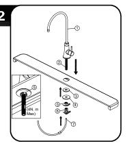
Place faucet (1) through the hole in countertop. Secure the faucet (1) to the countertop using the rubber washer (3) and the metal washer (4) provided, Tighten the nut (5), do not overtighten. Then tighten one end of the connector (6) joint at the bottom of the shank (2) and connect the other end to the pipe (7).
