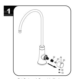
Shut off water supply. Remove index (1) and unscrew the set screw (2) on the handle (3). Remove handle (3) and loosen the screw (4) from valve stem. Loosen the inverter (5).
