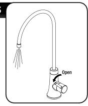
After installation is completed, turn on water supply, turn the handle in a counterclockwise direction. Flush the water lines for at least one minute.
