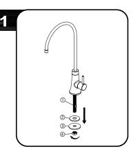
Before installation, shut off water supplies, remove old faucet. Remove the nut (4), metal washer (3) and rubber washer (2) from shank (1).
