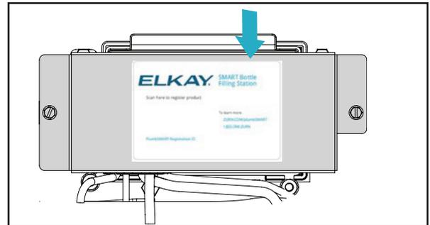
14. Install back bottle filler to the wall mounting plate and refasten using (2) screws making sure gasket is properly placed beneath the bottle filler.
