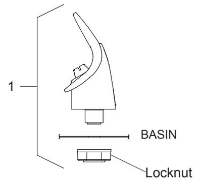
NOTE: WHEN INSTALLING REPLACEMENT BUBBLER AND PEDESTAL, TIGHTEN LOCKNUT ONLY TO HOLD PARTS SNUG IN POSITION. DO NOT OVER TIGHTEN.
