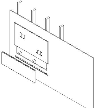
Includes the access panel and L-bracket for mounting. The access panel has a tab along the top which secures behind the fountain back panel. L-bracket is mounted to the wall. Access panel is secured to L-bracket with screws.
