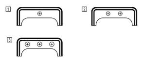
1-1/4" (32mm) Diameter Faucet Holes For 1 and 2 Hole Models 1-1/2" (38mm) Diameter Faucet Holes For 3 Hole Model Faucet Holes on 4" (102 mm) Centers
