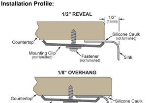
Designed to affix to the underside of any solid surface countertop
