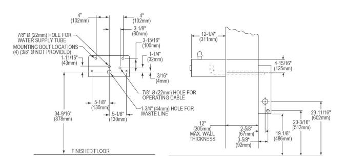
NOTE: ALL DIMENSIONS ARE TAKEN FROM THE FINISHED FLOOR ON THE SIDE OF THE WALL THAT THE FOUNTAIN IS ON
