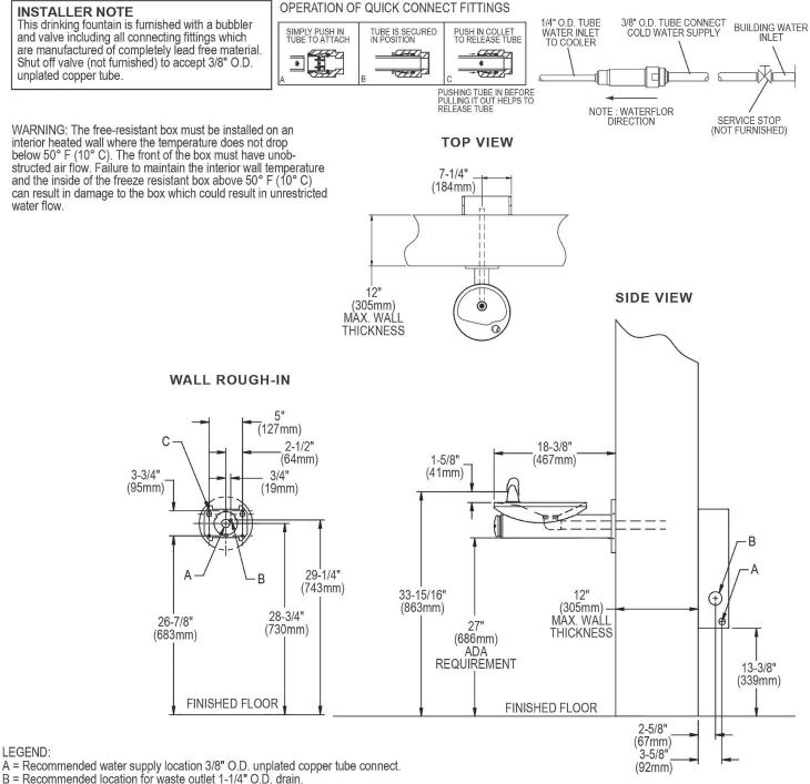
C = (4) Mounting holes 3/8" (10mm) dia. for securing fountain to wall.
