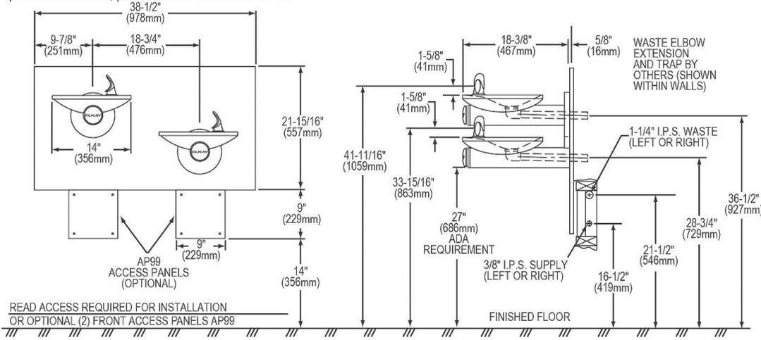
READ ACCESS REQUIRED FOR INSTALLATION OR OPTIONAL (2) FRONT ACCESS PANELS AP99
