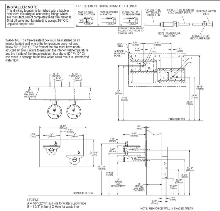
\*NOTE: ALL DIMENSIONS ARE TAKEN FROM THE FINISHED FLOOR ON THE SIDE OF THE WALL THAT THE FOUNAIN IS INSTALL ON.
