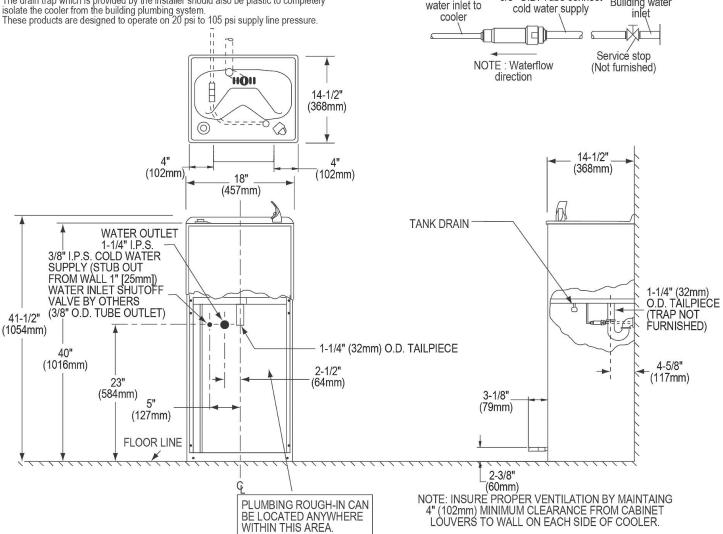
NOTE: New installations must use Ground Fault Circuit Interrupter (GFCI) It is highly recommended that the circuit be dedicated and the load protection be sized for 20 amps.
