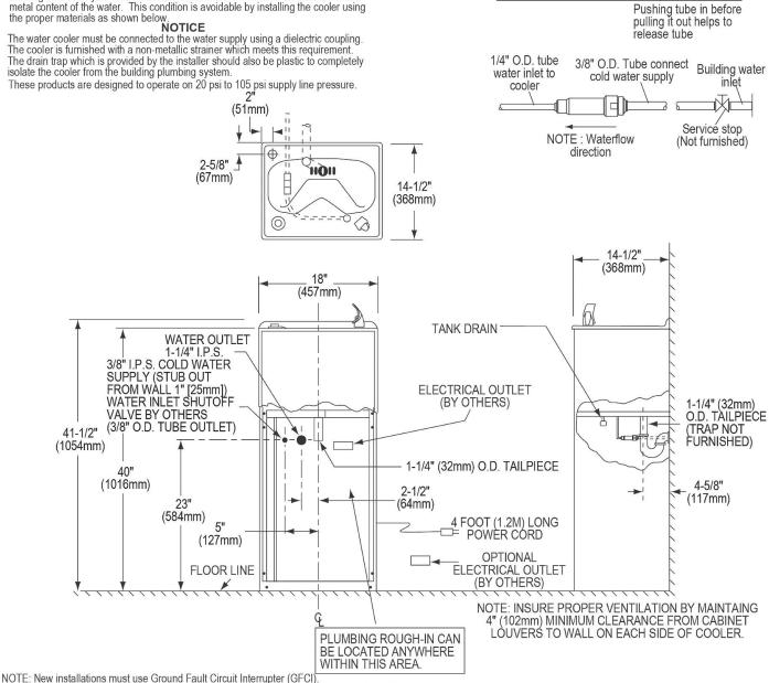
It is highly recommended that the circuit be dedicated and the load protection be sized for 20 amps.
