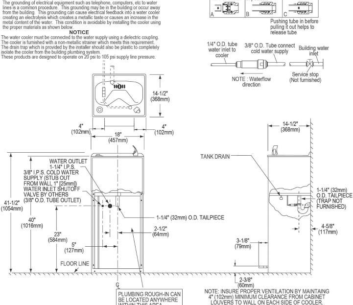
NOTE: New installations must use Ground Fault Circuit Interrupter (GFCI) t is highly recommended that the circuit be dedicated and the load protection be sized for 20 amps.
