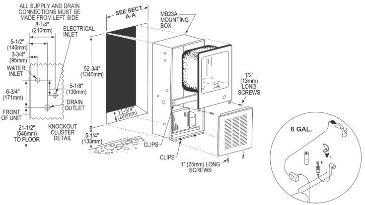
NOTE: New installations must use Ground Fault Circuit Interrupter (GFCI). It is highly recommended that the circuit be dedicated and the load protection be sized for 20 amps.
