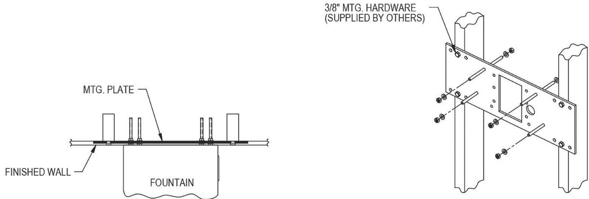
NOTE - AFTER INSTALLATION, THREADED RODS MAY NEED TO BE TRIMMED.
