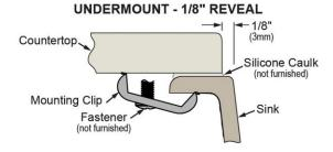
Designed to affix to the underside of any solid surface countertop.
