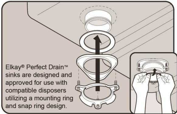
Elkay® Perfect Drain™ sinks are designed and approved for use with compatible disposers utilizing a mounting ring and snap ring design.
