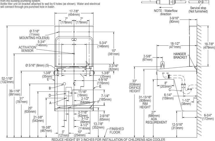
A = Recommended Water Supply location. Shut-off Valve (not furnished) to accept 3/8" O.D. unplated copper tube. Up to 3" (76mm) maximum out from wall.
