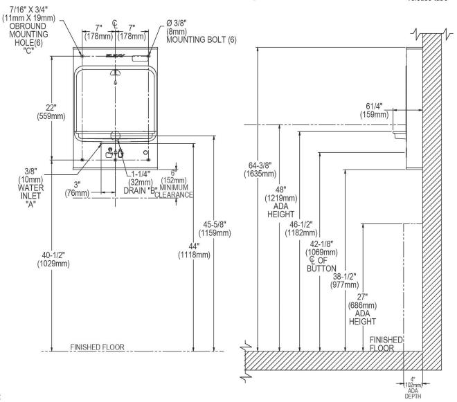
A = Recommended water supply location; 1/2" IPS maximum pipe size. Service stop valve not furnished.
