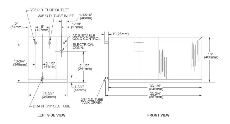
**NOTE:** This unit is intended for remote installation only. It is important to insure proper ventilation. Allow a minimum clearance of 6"(152mm) in front and 6"(152mm) in the rear of unit.
