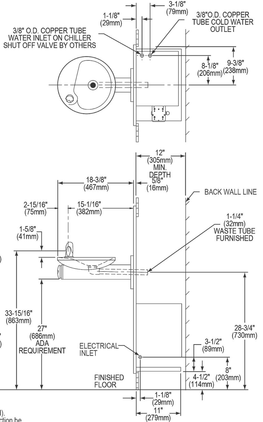
NOTE: New installations must use Ground Fault Circuit Interrupter (GFCI). It is highly recommended that the circuit be dedicated and the load protection be sized for 20 amps.
