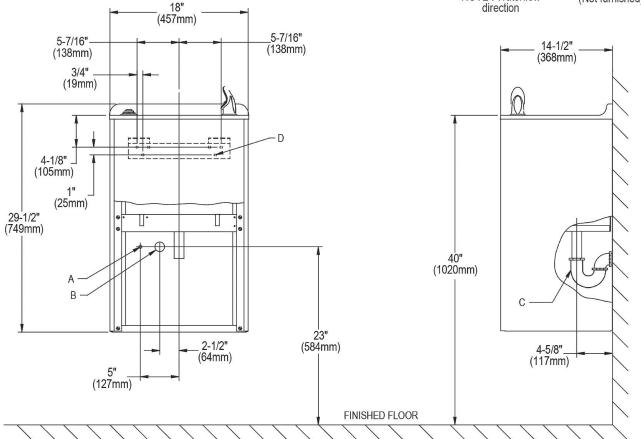
**LEGEND** A = Recommended water supply location 3/8" O.D. unplated copper tube connect stub out 1-1/2" (38mm) out from wall shut off by others.
