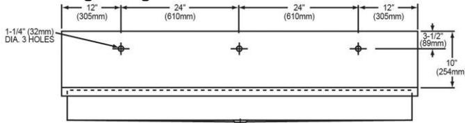
**Included with Product:** EWMA7220 sink, three LKB722C sensor faucets AC plug-in / 12 AA batteries, three LK723 thermostatic mixing valves, one LK18B grid drain
