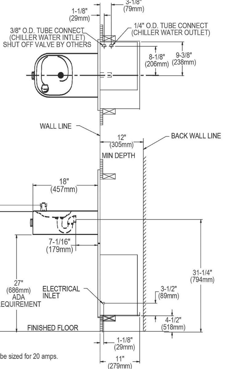
Note: New Installations Must Use Ground Fault Circuit Interrupter (GFCI).
