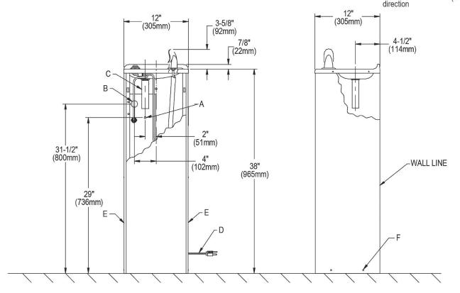
A = Recommended water supply location. Shut off valve (not furnished) to accept 3/8" O.D. unplated copper tube connect.
