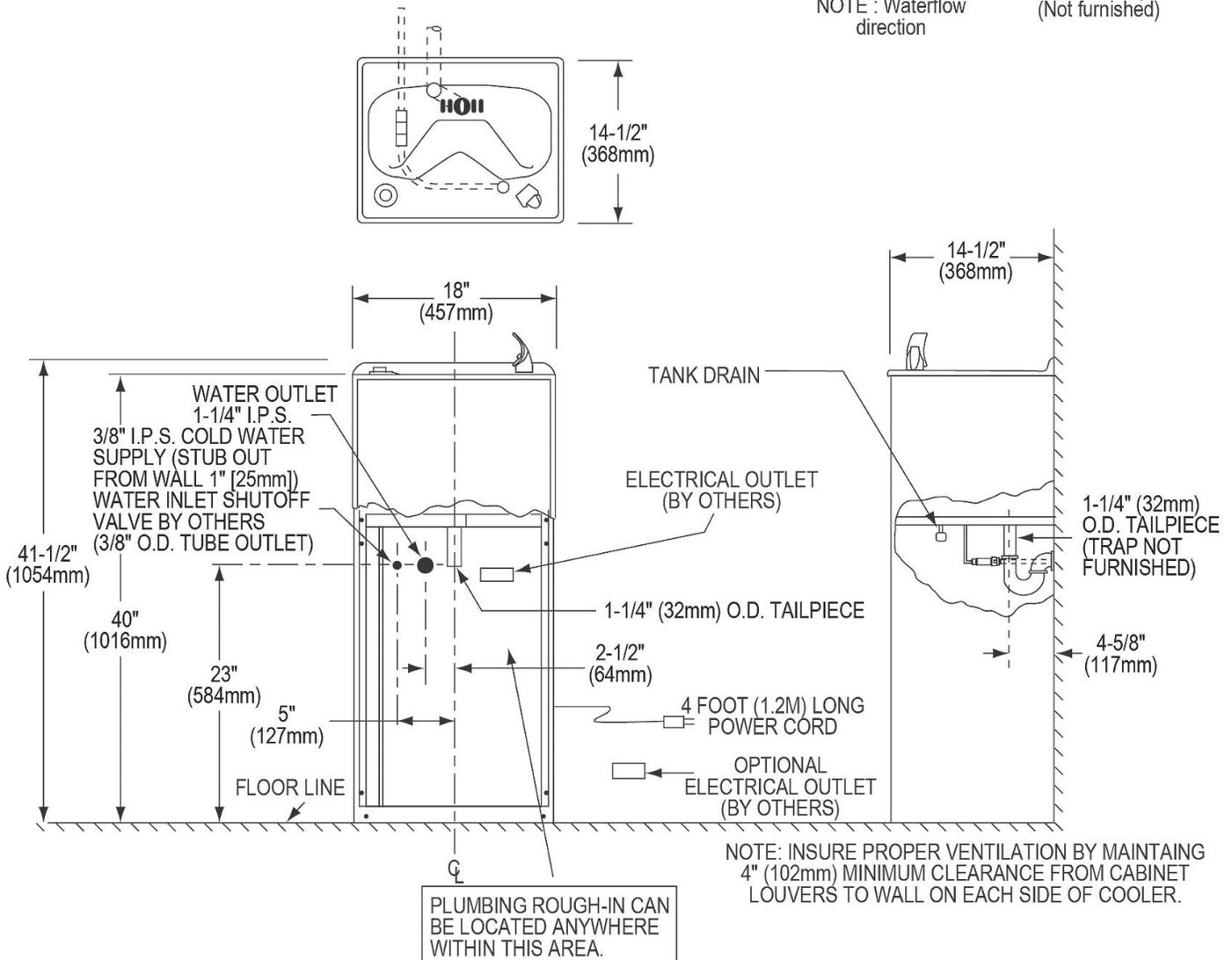
NOTE: INSURE PROPER VENTILATION BY MAINTAINING 4" (102mm) MINIMUM CLEARANCE FROM CABINET LOUVERS TO WALL ON EACH SIDE OF COOLER.
