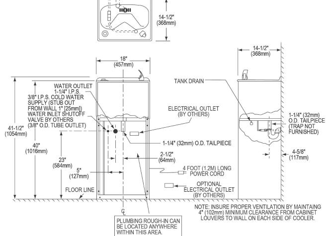
NOTE: New installations must use Ground Fault Circuit Interrupter (GFCI). It is highly recommended that the circuit be dedicated and the load protection be
