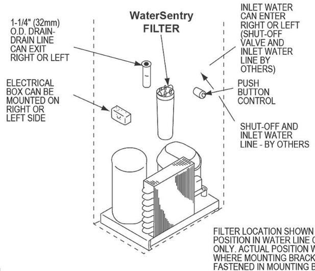
NOTE: New installations must use Ground Fault Circuit Interrupter (GFCI). It is highly recommended that the circuit be dedicated and the load protection be sized for 20 amps.
